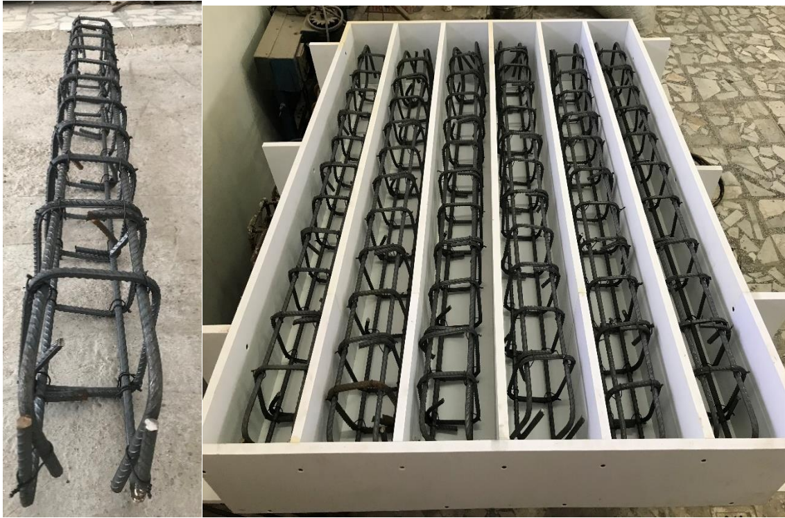
Figure 3. Fabrication of models for RFGPC beams
