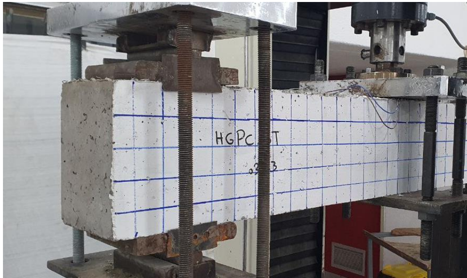
Figure 6. Test setup (Universal testing machine) and FRGPC beam specimen.
