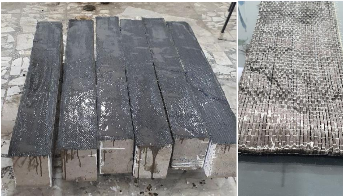
Figure 12. Damaged concrete beams strengthened with FRP sheets before testing, showing close-up of FRP mesh structure.
