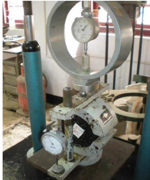
Fig 1.2 Marshall Test in Progress
