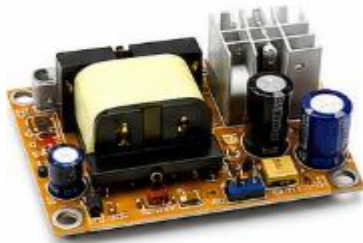
Fig 3 Power Supply Unit
