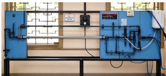
Figure 1. Setup of Double Pipe Heat Exchanger test rig
