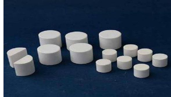
Fig. 1.1: Picture of the cylindrical pellets produced from pressing the milled and calcined powders.
